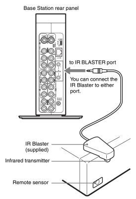
With reference to the operating instructions of the video devices, make sure to place the IR Blaster just above or below the remote sensor. Remote sensors on Sony Recorders and other products are identified by the 🖫 symbol.
